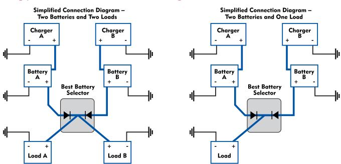
During normal operation, current to either a single load or dual loads flows from both chargers and both batteries through the BBS. Should one battery fail (e.g. shorted cell or open circuit) the other battery will continue to power one or both loads automatically and without interruption. The Best Battery Selector (BBS) OR diodes fully isolate a bad battery from the rest of the system.
